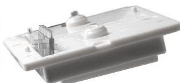
Figure 5: LED light pipes incorrectly installed
